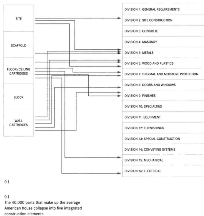
Figure 4b: Loblolly House component hierarchy. Kieran and Timberlake’s reorganization of the American house into five integrated assemblies collapses CSI MasterFormat’s divisions into a coordinated, offsite-ready system.
